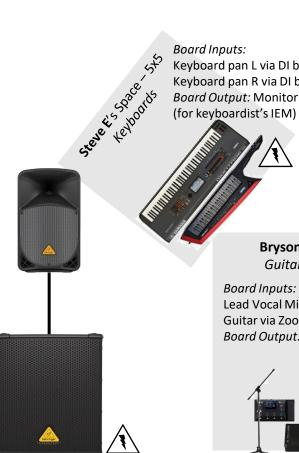
Keyboard pan L via DI box (XLR) Keyboard pan R via DI box (XLR) Board Output: Monitor Mix #2 (XLR)
